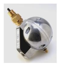
The condensate is accumulated in the reservoir of the device; when a prefixed level is reached, a leverism activated by the float opens the drain valve; the condensate is drained and the float comes back down and close the valve when a small amount of condensate is still in, to avoid waste of compressed air.
